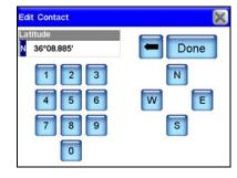
The Latitude entry is highlighted in the Edit Contact screen, at left. When Latitude is highlighted and selected it will bring up the Edit Contact screen keyboard for the Latitude entry, shown at right. You can use the keyboard to manually enter the latitude. The Longitude entry works the same way.
